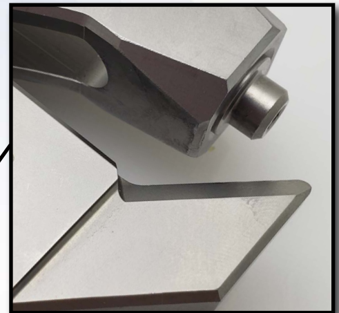
The jaw clamps down onto the modular hip stem, securing it in place for extraction.
